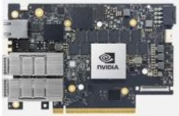
A photograph of a dual NVIDIA BlueField-3 DPU. The board is populated with various components, including a central chip with the NVIDIA logo, memory modules, and two QSFP112 ports on the left side. |
